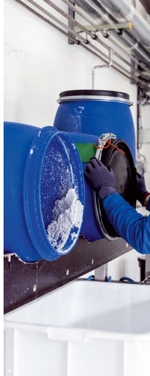
3, and 4 The raw mixture made from nitrocellulose comes from the Swiss site in Wimmis. In Aschau, it is first stored in a dedicated building to allow it to settle before undergoing further processing.
