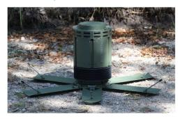
Weighing around 25 kilos, the ADW is 234 millimetres in diameter and features a launch-hardened design. It can be emplaced by hand or from logistic vehicles, via mine dispenser system or rocket artillery. Thanks to its networked communications, it can be activated, deactivated or reactivated, and reprogrammed so that it acts as an obstacle solely for enemy forces.
