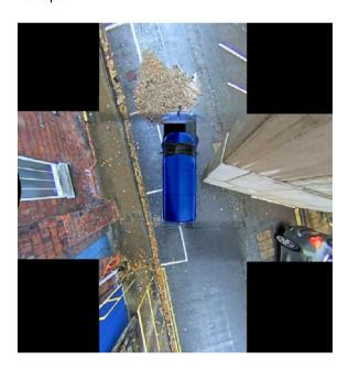
REUK's OVERVIEW combines images from several high specification sensors located around the vehicle for an optimum view of the surrounding environment, as if from directly above.
