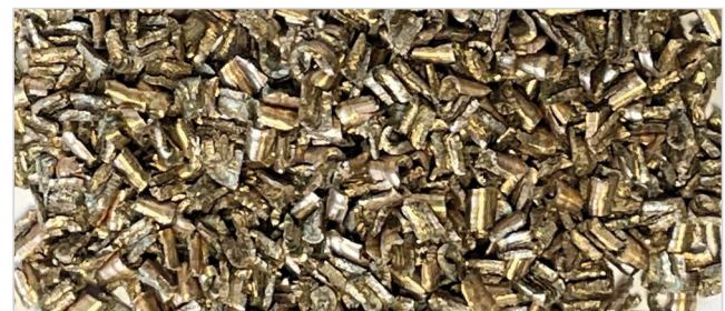
Fig. 6: EC7 chip with industrial machining
