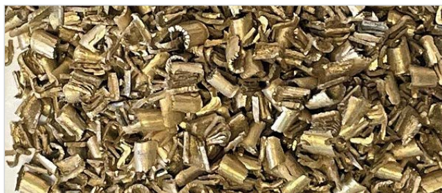
Fig. 5: Rg7 (CC493K) chip with industrial machining
