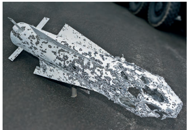
The tungsten alloy sub-projectile payload of the Oerlikon Ahead® round most effectively destroys the threat
