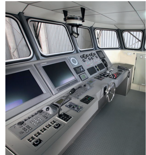
Integrated wheelhouse control console with all-round visibility
