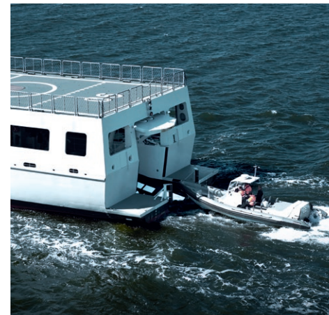
RHIBs are launched from the sides or via a stern ramp
