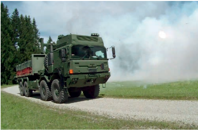
ROSY protecting the High Mobility Truck System HX77 of Rheinmetall MAN Military Vehicles
