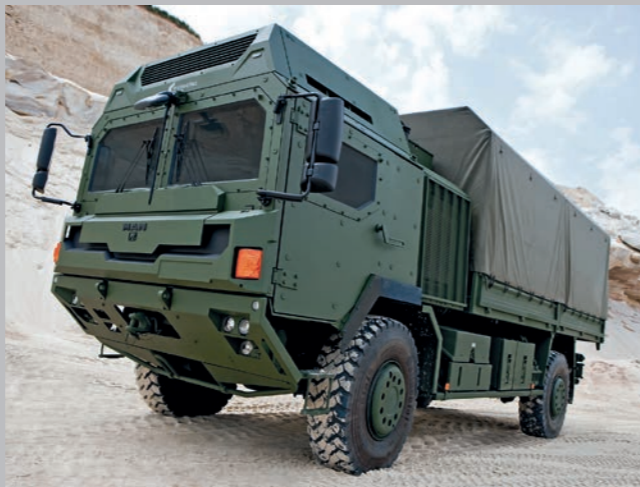
Concept B – Steel Cabin with Add-on-Armour for ballistic and mine/IED protection
