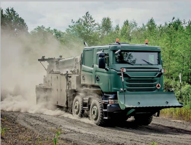
Concept A – Soft Skin Cabin with Armour Kit as Stand-alone inside Cabin
