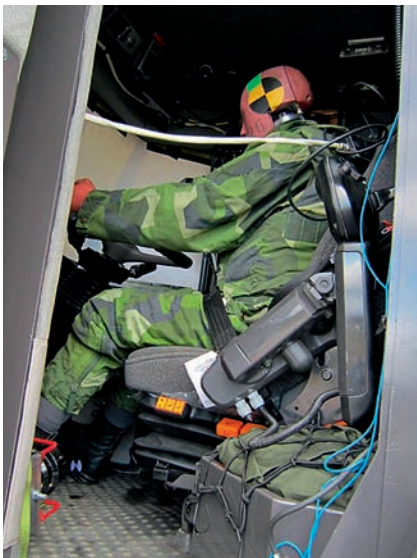
Mine blast test on excavator
