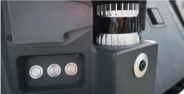
Connected to a set of advanced sensors such as LiDAR, radar, and cameras, the PATH technology is designed to convert any drive-by-wire platform into an autonomous vehicle
