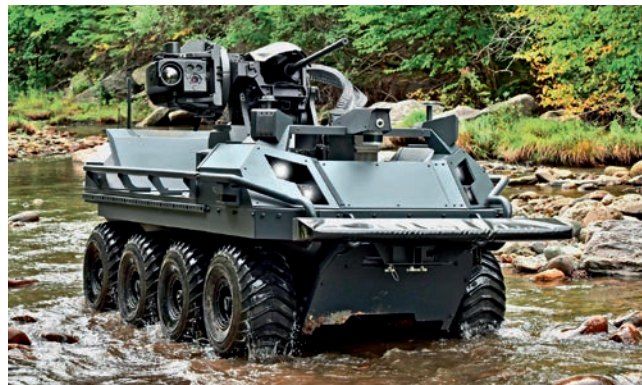
Mission Master SP – Fire Support equipped with Rheinmetall Fieldranger Multi remotely controlled weapon station
