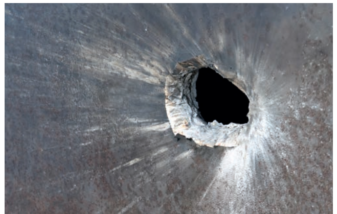
35 mm steel armour plate penetrated by an unprogrammed Ahead round (target angle 45°/target distance 500 m)
