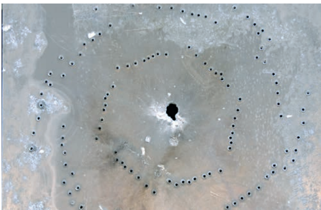
Pattern of one Ahead round, shot through a 20 mm aluminium plate
