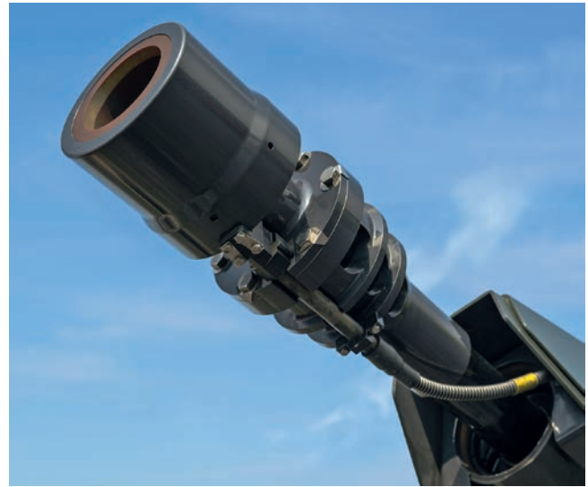
Ahead muzzle velocity measuring and programming base
