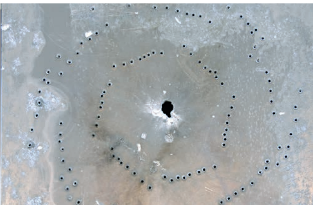
Pattern of one Ahead round, shot through a 20 mm aluminium plate
