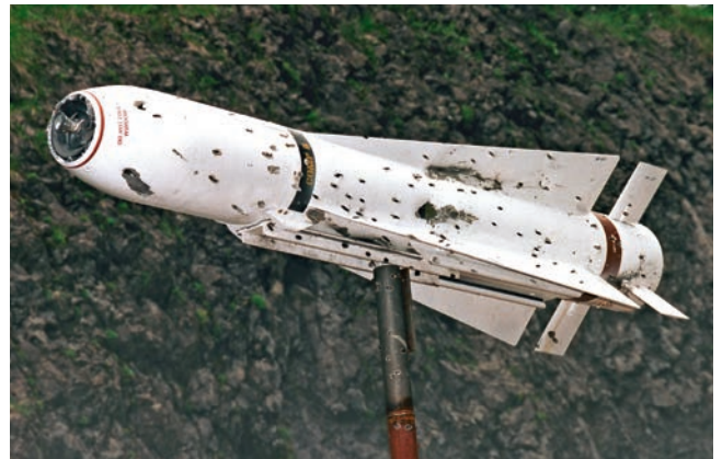
Air-to-ground missile destroyed by one burst of Ahead ammunition
