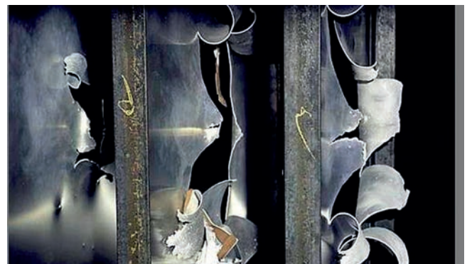
FAP fragments cause massive structural damages deep inside the target
