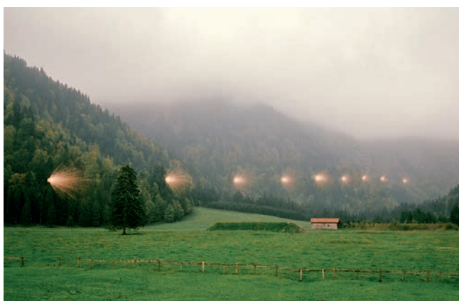
10 rounds of Air Burst Munition – precise release of tungsten carbide sub-projectiles
