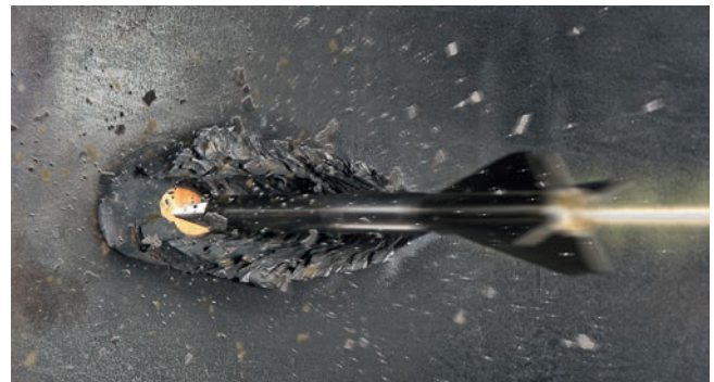
35 mm x 228 APFSDS-T against single RHA-plate at a distance of 2 km
