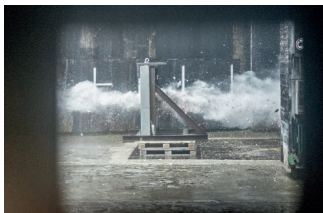
30 mm x 173 KETF against 20 cm double reinforced concrete – engagement in depth
