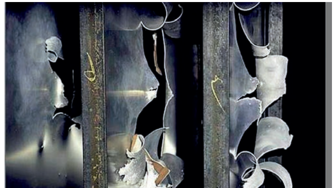
FAP fragments cause massive structural damages deep inside the target
