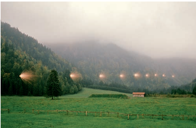
10 rounds of Air Burst Munition – precise release of tungsten carbide sub-projectiles
