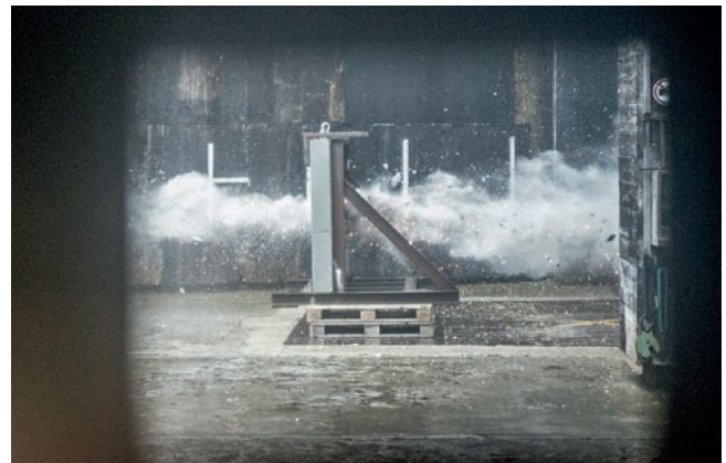
30mm x173 KETF against 20cm double reinforced concrete – engagement in depth
