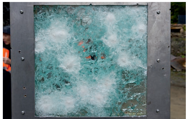
Air Burst Munition against armoured glass
