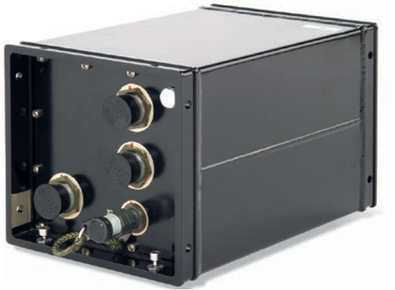
ABM electronics (Puma): 296 x 192 x 180 mm, 5.5 kg
