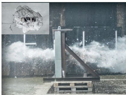
30 mm x 173 PMC308 KETF against 20 cm double reinforced concrete in unprogrammed mode
