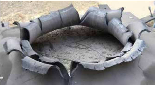
Main charge effect against 20mm steel target
